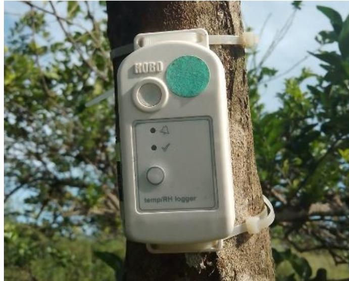
Figura 2. Sensor HOBO MX2301A.
